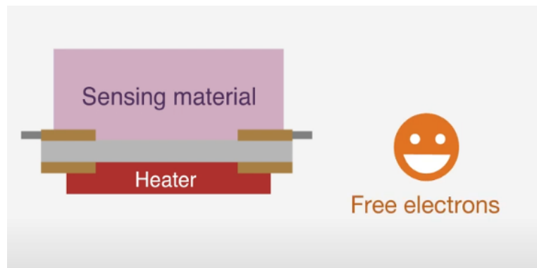
Figure 2.2. Metal Oxide Gas Sensor Structure (Figaro, 2020)
