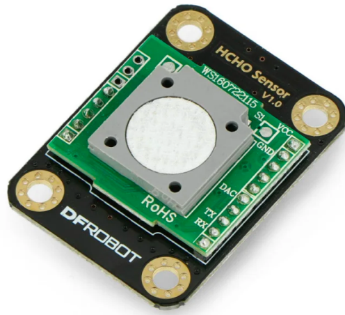
Figure 3.10. DFRobot Gravity HCHO Sensor (Gravity, 2021).
